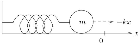
FIGURE 1. one-dimensional harmonic oscillator
