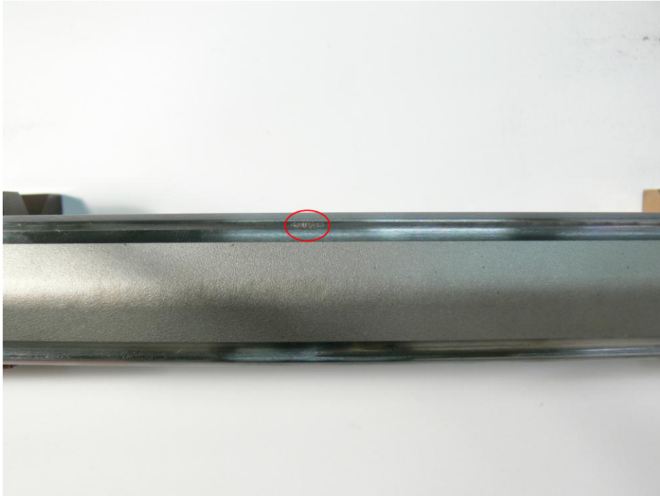
Fig 11 Flaking of shaft raceway
