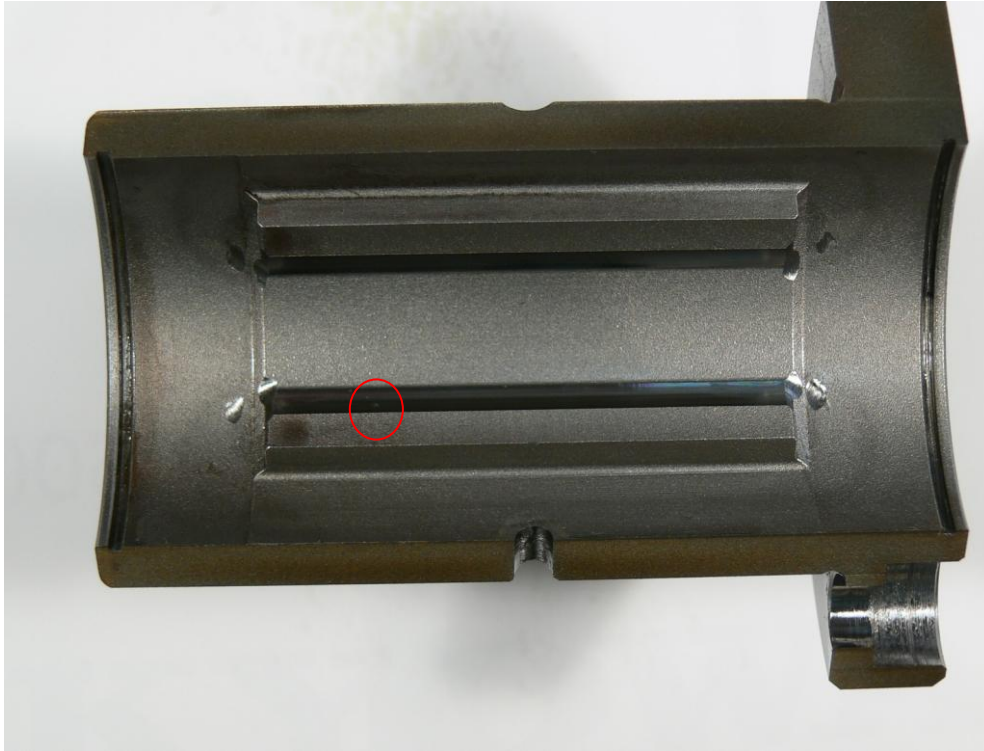
Fig 9 Flaking of nut raceway
