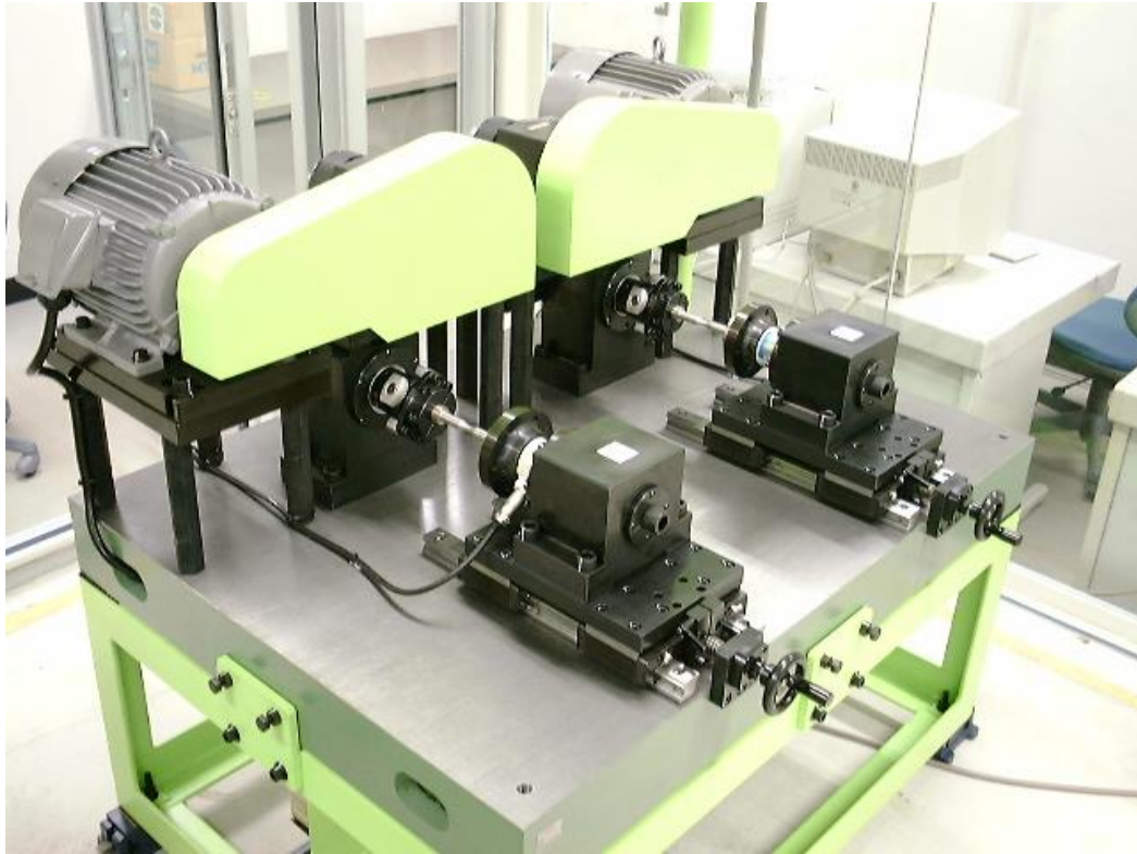
Fig.2 Alternating torsion life test rig
