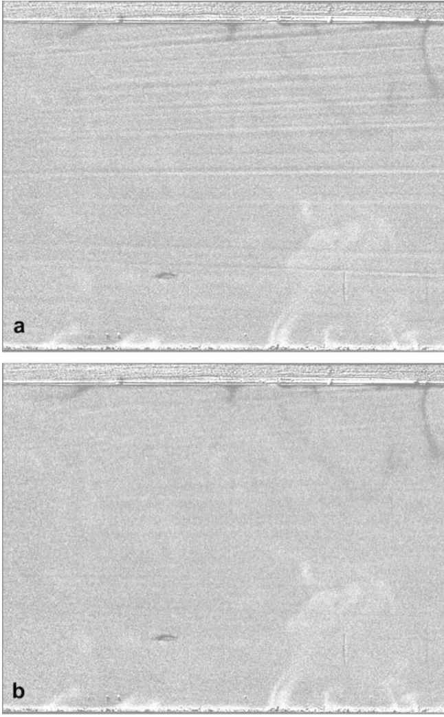
Fig. 4. Ratio of fluorescence intensity; a without blurring compensation, and b with blurring compensation
