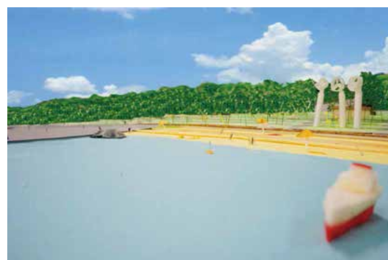
Model of a gradual seawall of 6.5m high by residents suggestion
