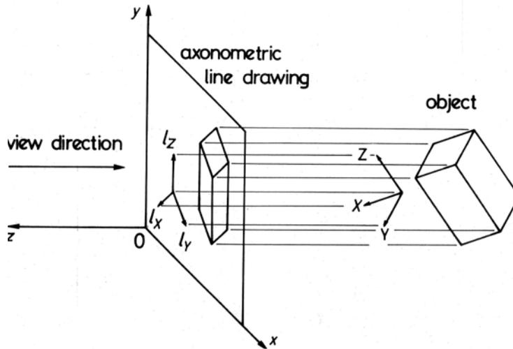
Figure 5.8. Axonometric projection.
